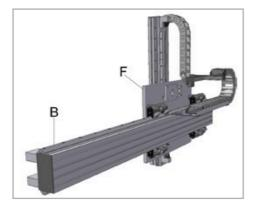
To replace a prismatic guide (B), ensure that the bearings which slide over them are discharged: for this reason, in the case of a guide on the horizontal axis, it is necessary to support the main plate or the carriage (F), so that its weight and all the equipment mounted on board, doesn't rest on bearings.
