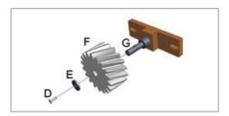
**e.** Before axis commissioning, make sure that the lubrication pinion is soaked with grease again.
